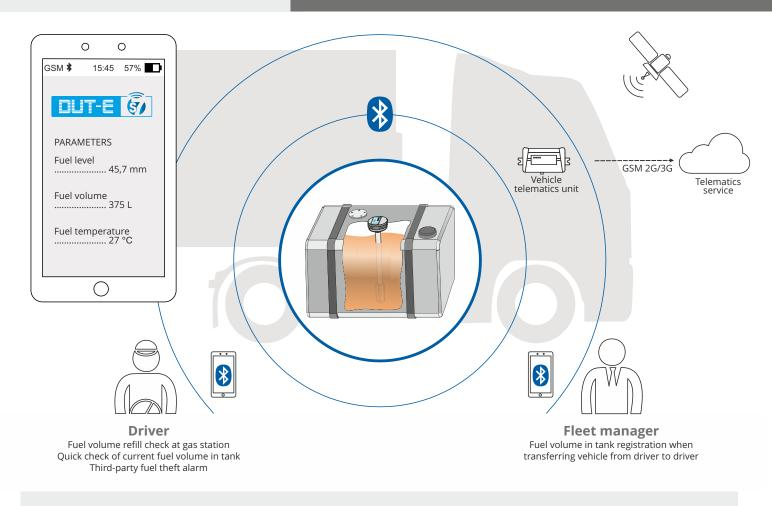
DUT-E S7 transmits data on fuel level/volume simultaneously to several devices: telematics unit, smartphones, tablets.
