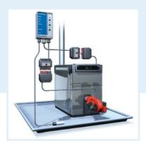
Application For visual and audible alarms in the event of accumulations of liquids below the burner of an oil fuelled system and for switching off the burner in alarm conditions. Suitable for the following media: water, fuel oil EL, L M and diesel fuel.
