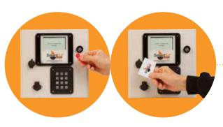
Touch the authorised vehicle ID key, fob or NFC card onto the sensor of the unit
