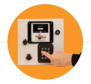
Once authorised, the unit can request the vehicle speedo/hourmeter reading and/or job number, which helps with scheduling maintenance
